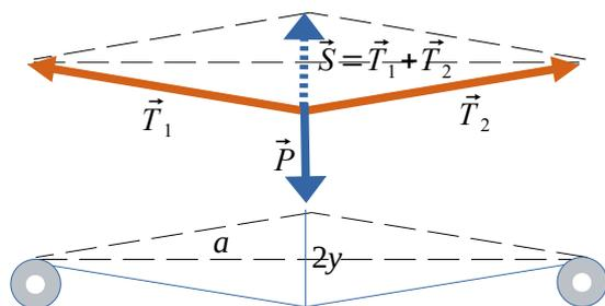
$$T_1 = T_2 = T = Mg$$
